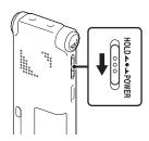
Slide the HOLD/POWER switch in the direction of "POWER" for more than 1 second. The IC recorder is turned on, and "Accessing..." is displayed.
